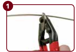
Trim cable to length
